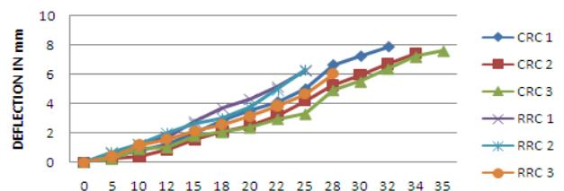
Fig. 8: Load deflection curve for control and retrofitted beam
