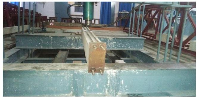
Fig. 6: Typical view of loaded retrofitted beam
