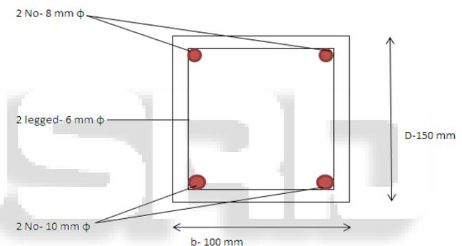
Fig. 2: Beam cross section
