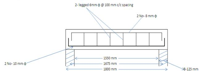
Fig. 1: Beam elevation
