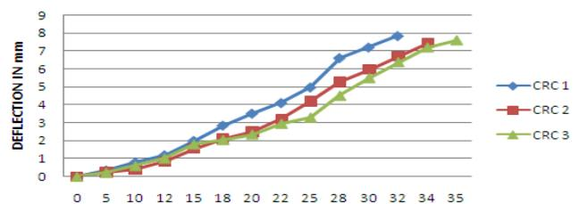
Fig. 7: Load deflection curve for control beam
