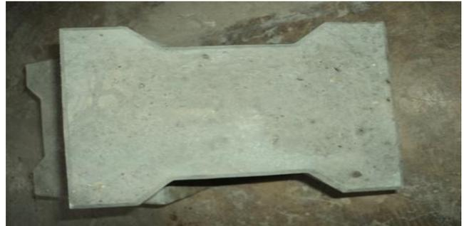
Fig. 3: Cross Section of Concrete Paver Block specimen after Curing
