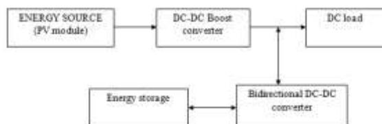
Fig. 1: Bidirectional DC-DC converter in renewable energy storage systems
