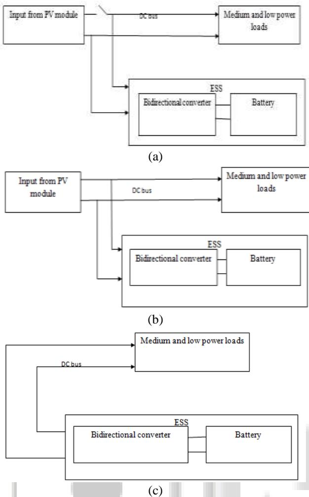
Fig. 2: Block diagram of (a) PV system with ESS (b) ZETA mode (c) SEPIC mode
