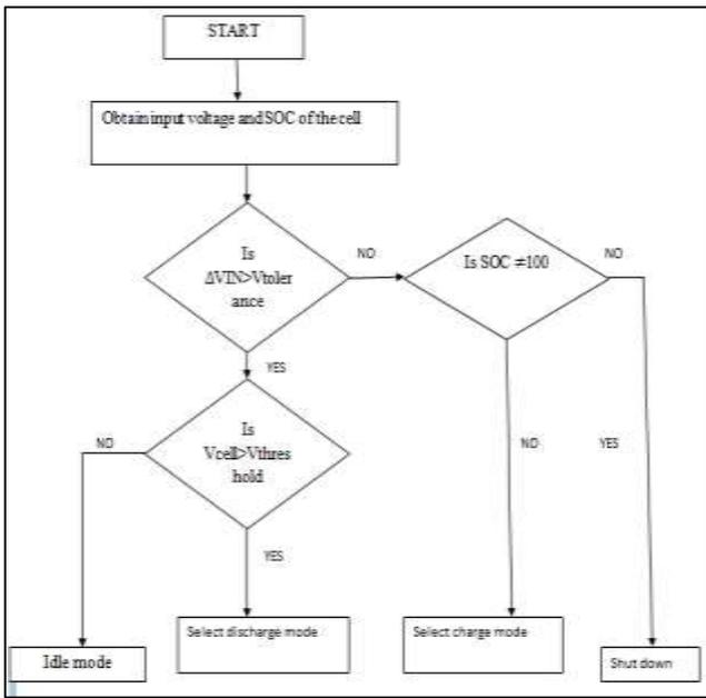
Fig. 5: Flow chart of mode selection algorithm
