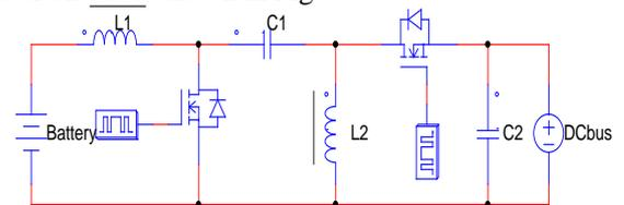
Fig. 4: Circuit diagram of coupled inductor based sepic/zeta converter
