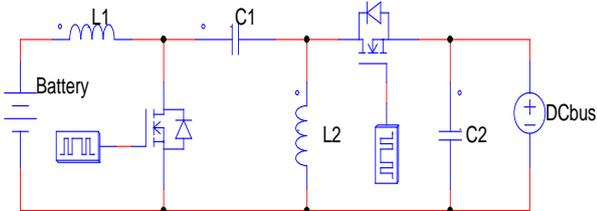
Fig. 3: circuit diagram of conventional sepic /zeta converter
