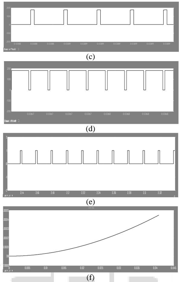
Fig. 7: Simulation results for zeta mode: a) input voltage b) output voltage c) voltage across Sepic switch d) voltage across Zeta switch e) switching pulses for Zeta switch f) battery state of charge (SOC)
