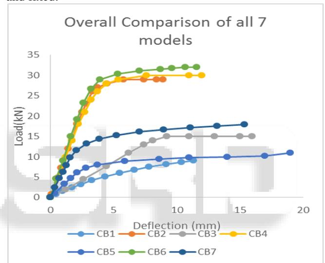
Fig. 12: Overall Comparison of Circular web openings
