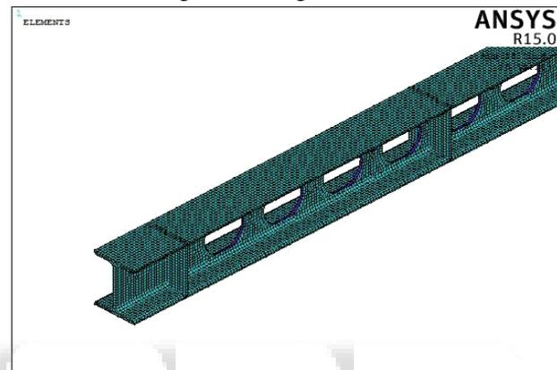
Fig. 3: Meshing of Beam
