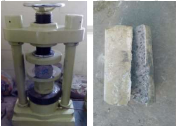
Fig. 7: Splitting Tensile Strength Test
