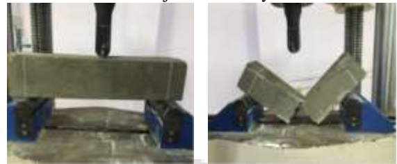
Fig. 9: Flexural Strength Test
