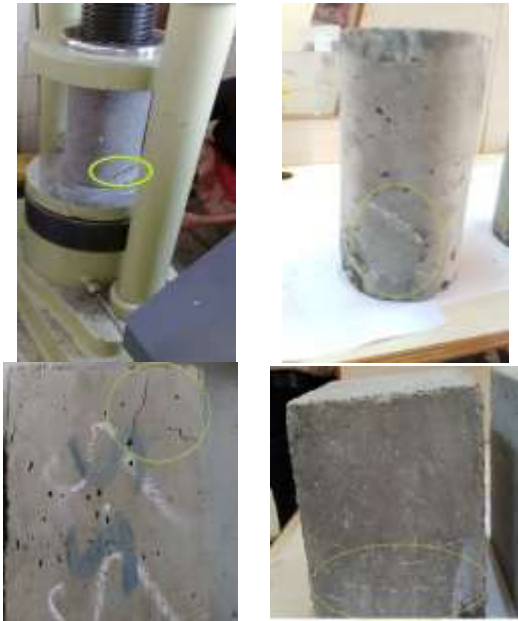
Fig. 11: Healing Mechanism of Cube and Cylinders
