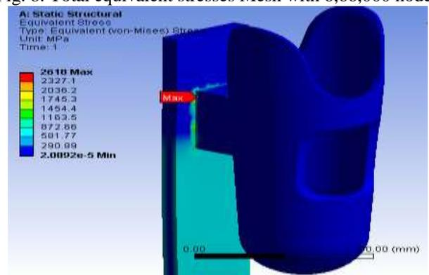
Fig. 9: Total equivalent stresses Mesh with 6,66,000 nodes
