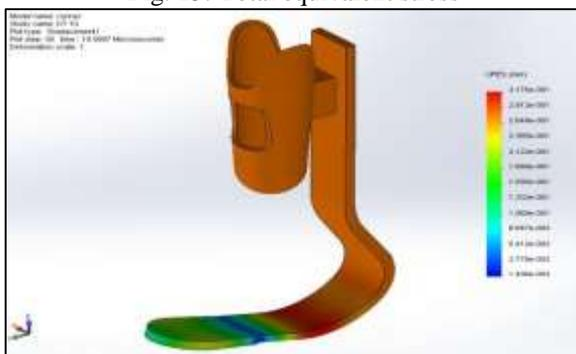
Fig. 16: Total deformation
