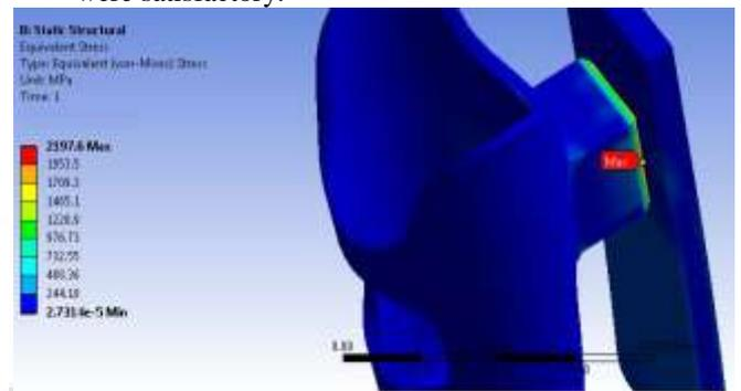
Fig. 7: Total equivalent stress: Mesh with 11,496 nodes
