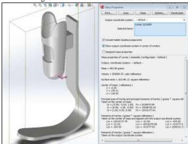
Fig. 6: Mass properties defined in Solid works
