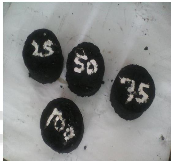
Fig. 3: Specimen prepare by replacing cement with fly ash in the order 25%, 50%, 75% and 100%
