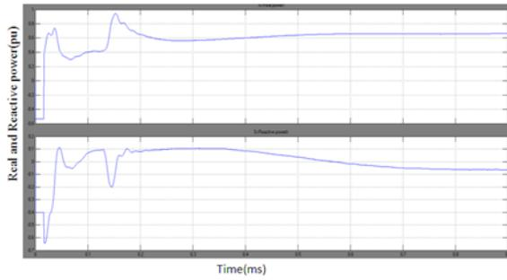
Fig. 7: Simulation result of DFIG Real and Reactive power without STATCOM.
