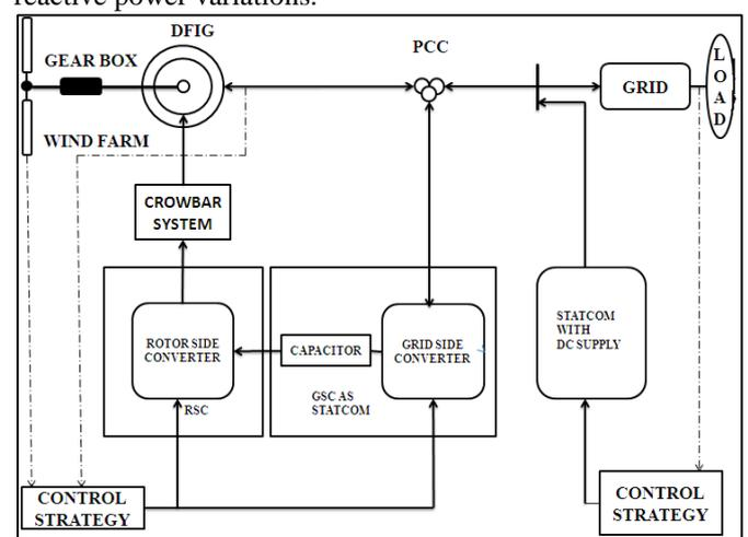
Fig. 1: DFIG with RSC-GSC control
