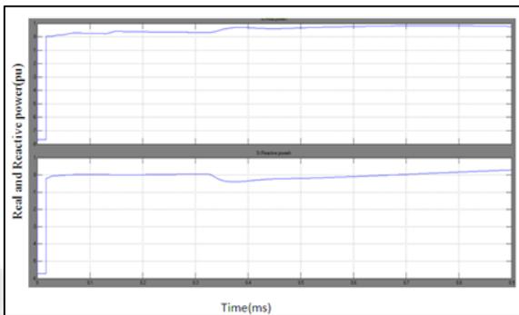
Fig. 8: simulation result of DFIG real and reactive power with STATCOM.
