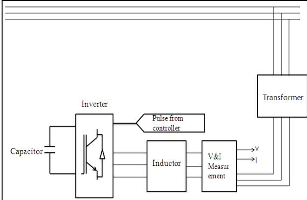
Fig. 4: STATCOM with Grid Connection
