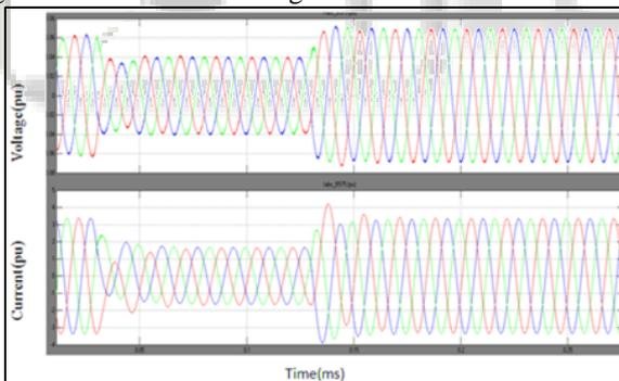
Fig. 9: simulation result of DFIG's grid input voltage.
