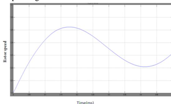
Fig. 10: simulation result of DFIG variable rotor speed.
