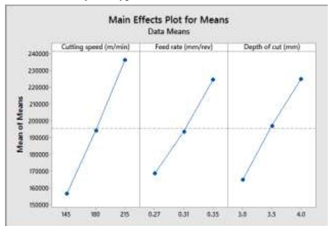
Fig. 1: Main effect plot for means for material removal rate of 'S' type Nitride ceramic insert
