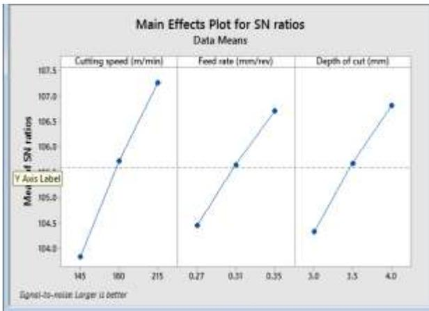
Fig. 2: Main effect plot for SN ratio for material removal rate of ‘S’ type Nitride ceramic type insert
