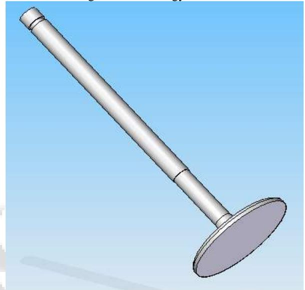
Fig. 4: Solid Edge image of conventional valve
