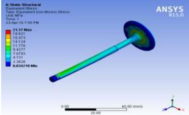
Fig. 14: Stress (21.17MPa) of face modified valve in different position
