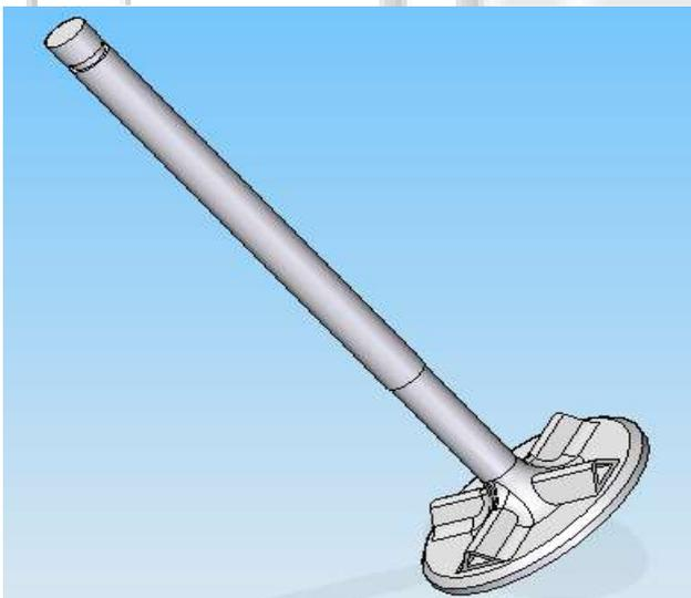
Fig. 16: Design of valve head modification
