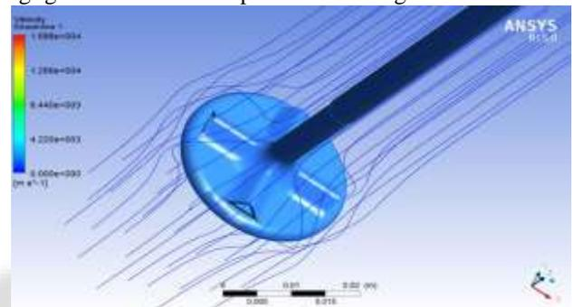
Fig. 18: The motion of charge flow around the valve in suction stroke
