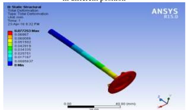
Fig. 19: Deformation (0.07725mm) of face modified valve in different position
