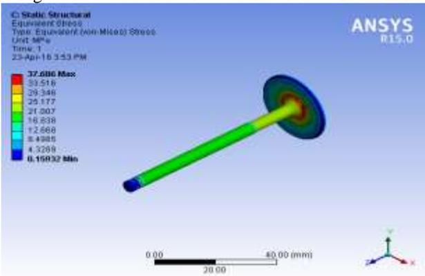
Fig. 8: The conventional valve stress is 37.686MPa
