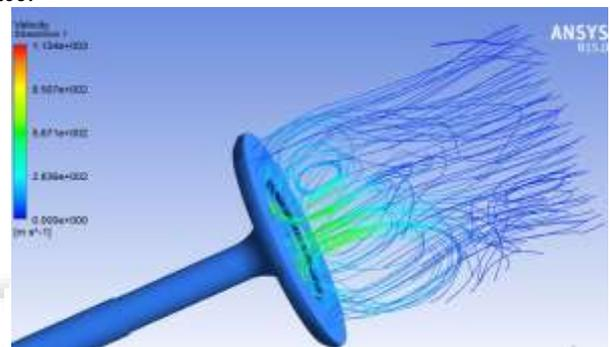
Fig. 11: Charge particle in swirl motion during compression stroke
