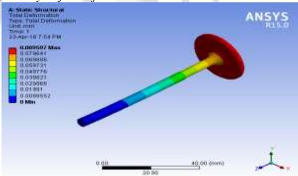
Fig. 12: Deformation (0.089597mm) of face modified valve in different position
