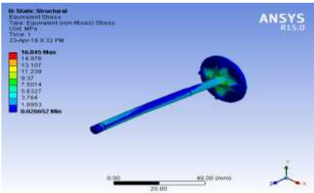
Fig. 20: Stress (16.845MPa) of face modified valve in different position
