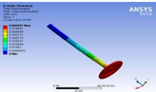
Fig. 13: Deformation (0.089597mm) of face modified valve in different position
