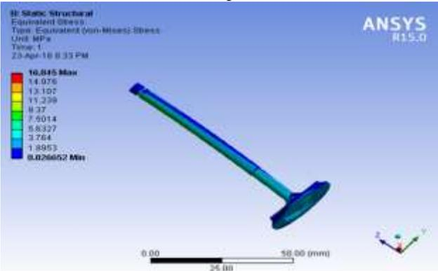
Fig. 21: Stress (16.845MPa) of face modified valve in different position
