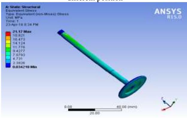
Fig. 15: Stress (21.17MPa) of face modified valve in different position
