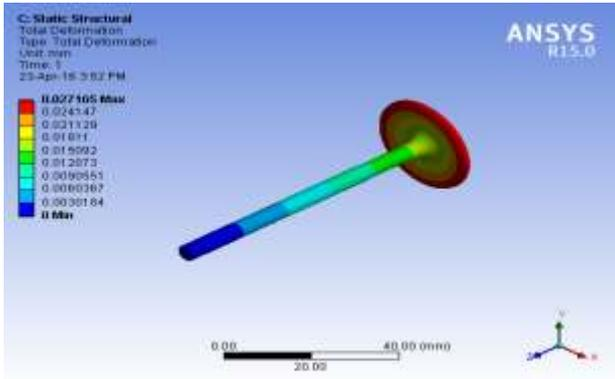
Fig. 7: Conventional valve deformation 0.027165mm
