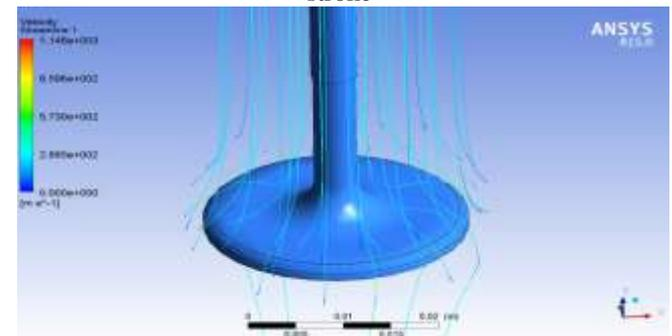
Fig. 6: The flow of charge entering during suction stroke
