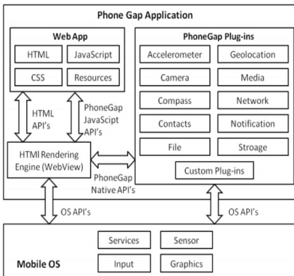
Fig. 2:- Complete schema of phone gap architecture.
