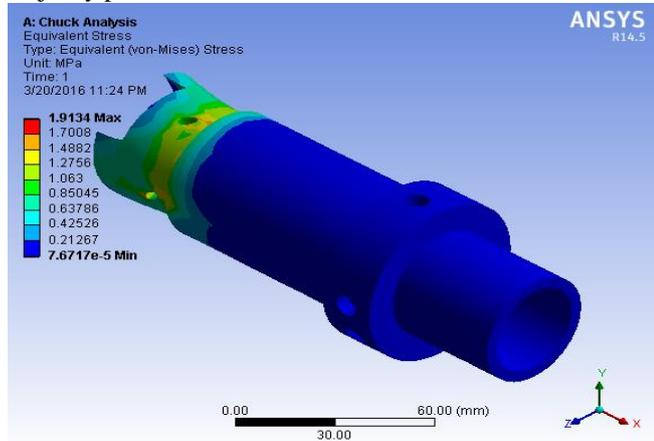
Fig. 7: Equivalent Stress
