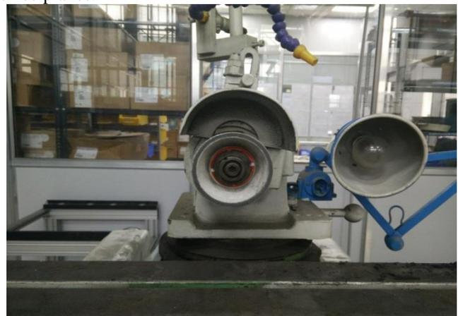
Fig .1: Grinder Wheel on Tool & Cutter Machine
