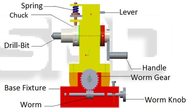
Fig. 6: Design of Fixture
