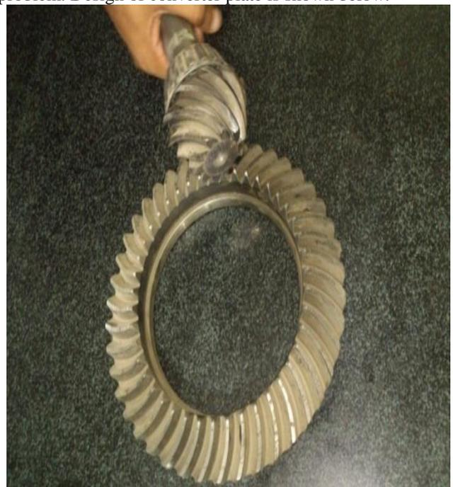
Fig. 1: Crown wheel and pinion
