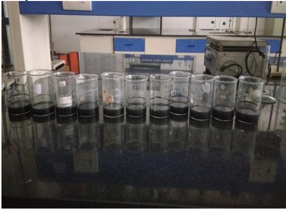
Fig. 1: Synthetic Groundwater Samples Mixed With Adsorbent
