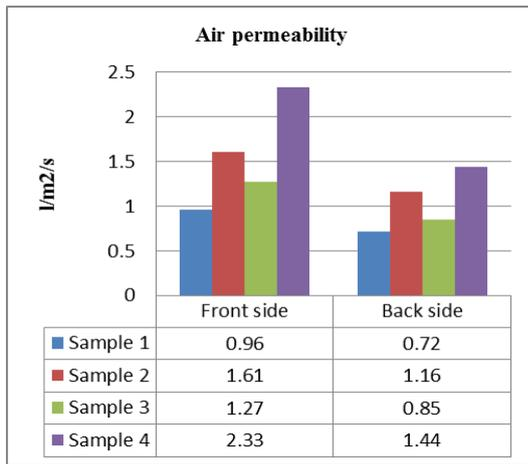
Fig. 2: Air permeability of samples.
