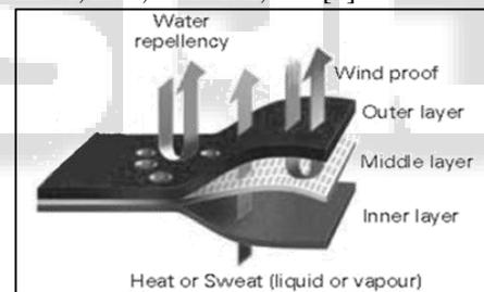
Fig. 1: Example of multilayered fabric used in sports shoes
