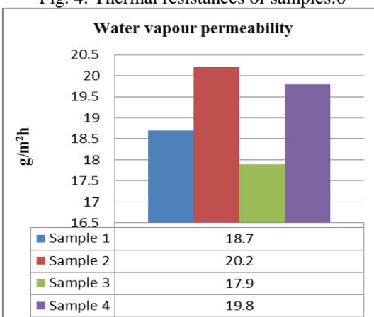
Fig. 5: Water vapour permeability of samples.
