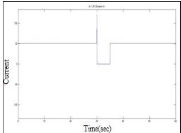
Fig. 2: Current through CB1 during Fault
