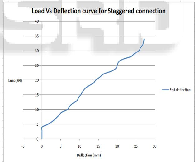
Fig. 4: Graph for staggered arrangement of bolts deflection
