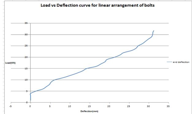
Fig. 5: Graph for linear arrangement of bolts deflection
