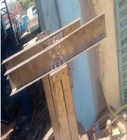
Fig. 1: Beam Column connections using Self Tapered Screws in staggered arrangement of bolts
