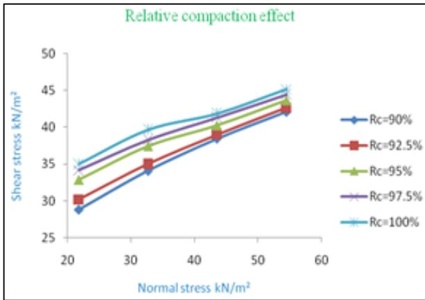
Fig. 5: Relative compaction effect
