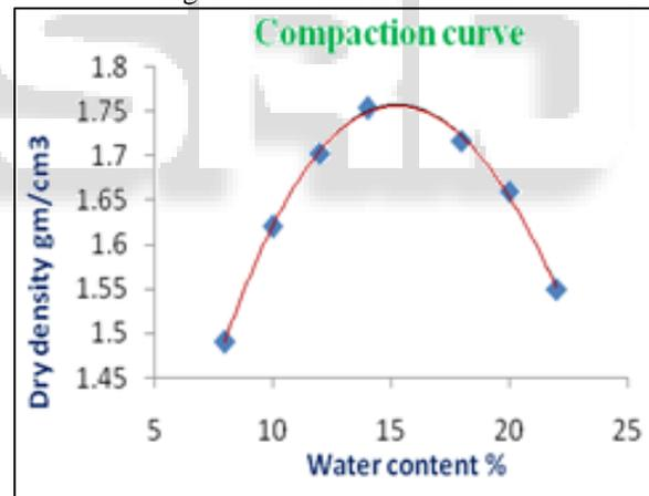
Fig. 2: Compaction curve
