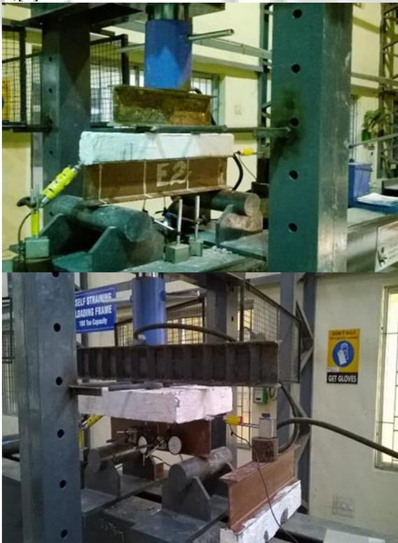
Fig. 6: Test setup for the composite beam
