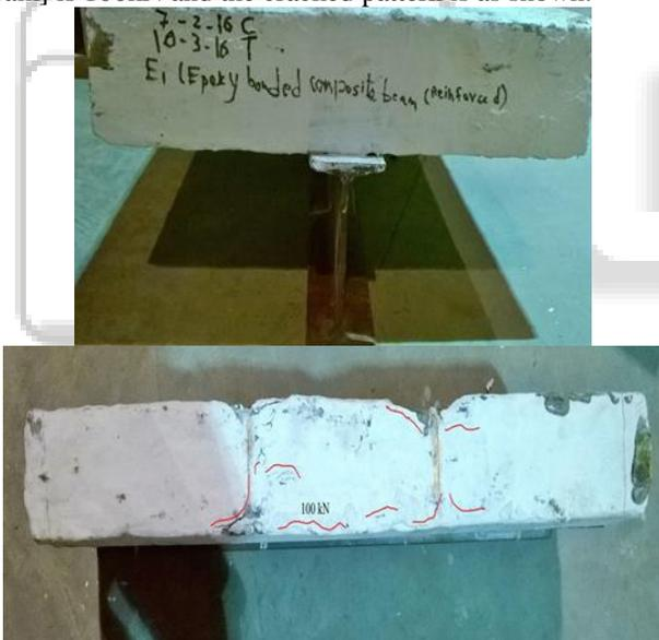
Fig. 8: Failure load of composite beam
