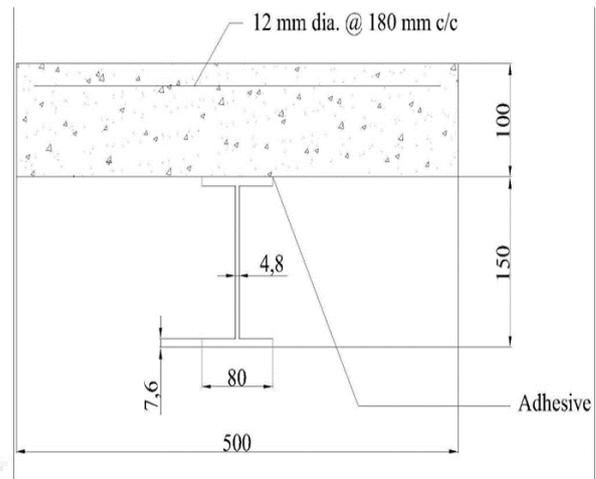
Fig. 2: Reinforcement details of composite beam
