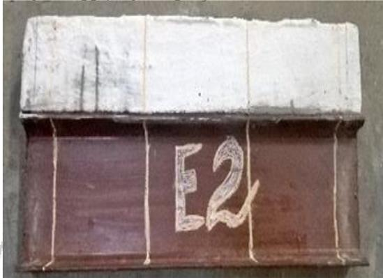
Fig. 5: After epoxy bonding
