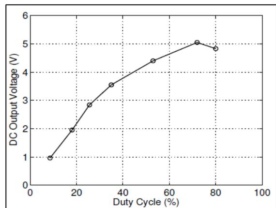
Fig. 4: The DC output voltage at various duty cycles
