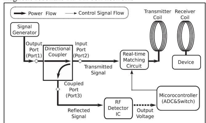
Fig. 1: Block diagram of the WPT system
