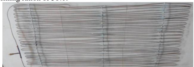
Fig. 1: Closed loop PHP
