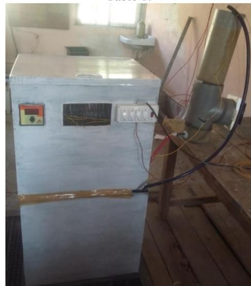
Fig. 6: Actual Experimental Setup for Heat Pipe Air Conditioning System
