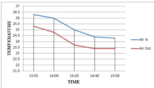
Fig. 7: Change in Temperature of Inlet and Outlet air with time for Indoor operating condition
