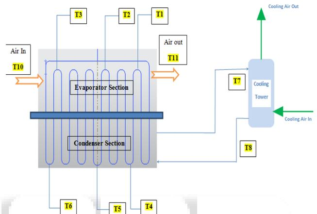
Fig. 5: Schematics of Heat Pipe Air-Conditioning Showing arrangement of all thermocouples
