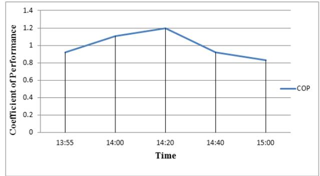
Fig. 8: Change in COP with time for Indoor operating condition
