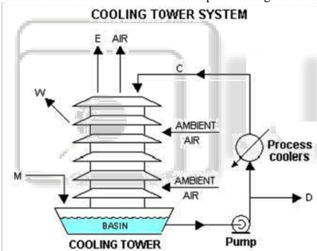
Fig. 3: Schematics Diagram of Cooling Tower
