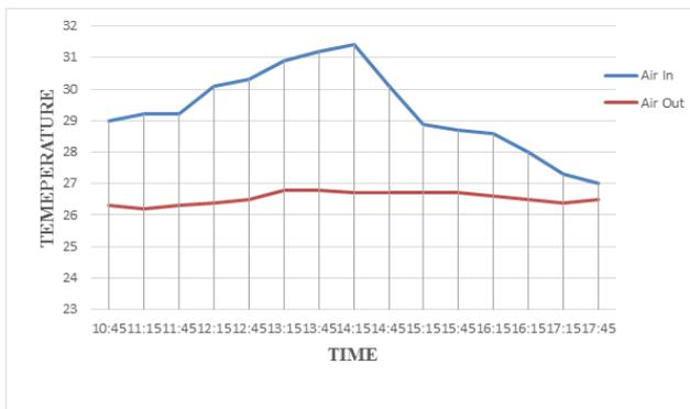
Fig. 11: Change in temperature of Inlet and Outlet air with time for Outdoor operating condition
