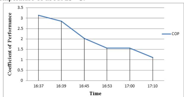
Fig. 10: Change in COP with Time for Window Operating Condition
