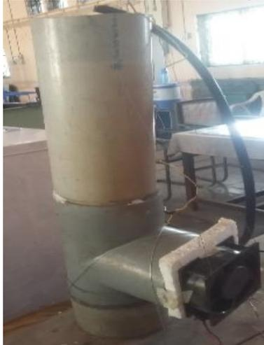
Fig. 4: Actual Cooling Tower observations. This is possible with help of digital temperature Indicator and Thermocouple wires.
