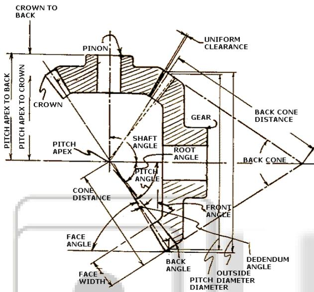
Fig. 5: Bevel-Gear Geometry
