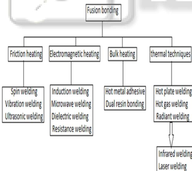
Fig. 7: Methods of welding thermoplastics
