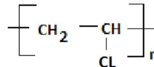
Fig. 5: Polyvinyl Chloride
