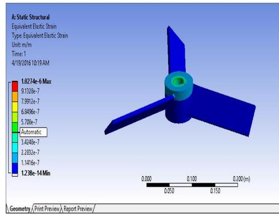
Fig. 6: Von misses strain in impeller.
