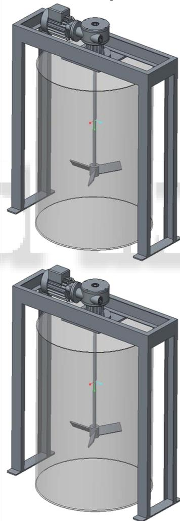
Fig. 1: Chemical Mixing Agitator Model.
