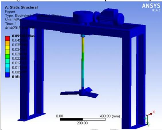
Fig. 4: Von misses stresses in impeller assembly.
