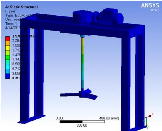
Fig. 3: Von misses strain in impeller assembly.
