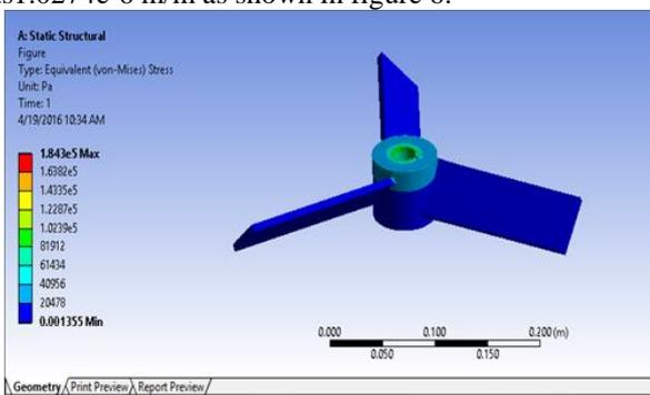
Fig. 5: von misses stresses in impeller
