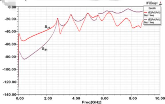
Fig. 11: NEXT and FEXT results obtained by using HFSS
