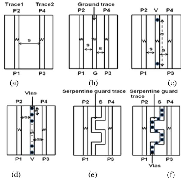
Fig. 1: Microstrip line geometry (a) Two conductor traces (b) Ground trace in between (c) Ground trace with 2 vias in between (d) Ground trace with 12 vias in between (e) Serpentine guard trace in between (f) Serpentine guard trace with vias in between
