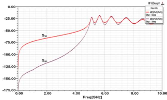
Fig. 9: NEXT and FEXT results obtained by using HFSS
