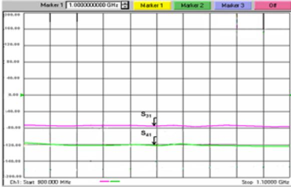
Fig. 10: Experimental results for NEXT and FEXT
