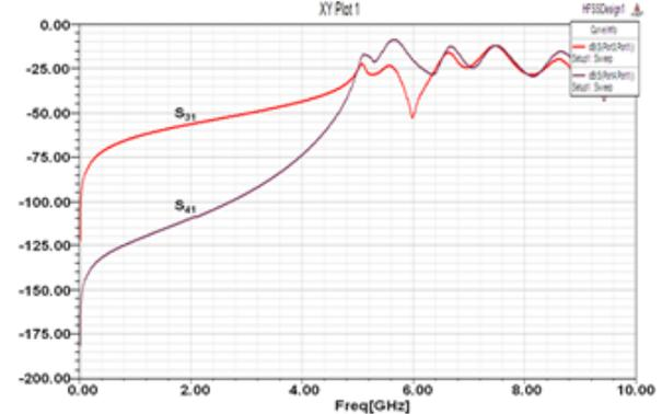
Fig. 13: NEXT and FEXT results obtained by using HFSS
