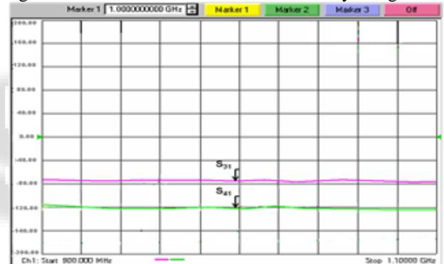
Fig. 14: Experimental results for NEXT and FEXT
