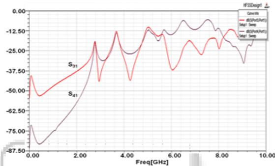
Fig. 3: NEXT and FEXT results obtained by using HFSS
