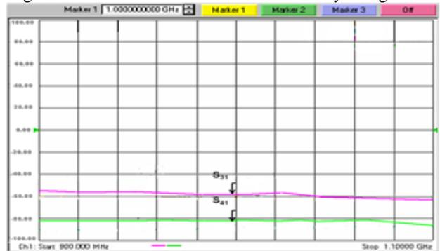
Fig. 8: Experimental results for NEXT and FEXT
