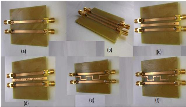
Fig. 2: Microstrip line geometry (a) Two conductor traces (b) Ground trace in between (c) Ground trace with 2 vias in between (d) Ground trace with 12 vias in between (e) Serpentine guard trace in between (f) Serpentine guard trace with vias in between
