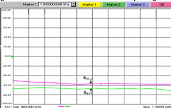
Fig. 12: Experimental results for NEXT and FEXT
