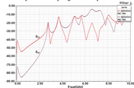
Fig. 5: NEXT and FEXT results obtained by using HFSS
