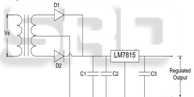
Fig. 1: Circuit diagram of constant voltage charger
