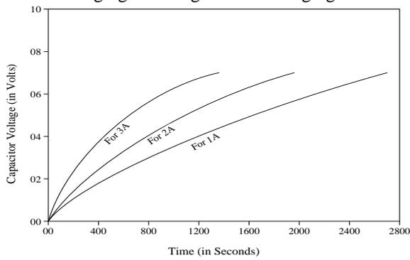
Fig. 3: Ultracapacitor charging graph for different charging currents
