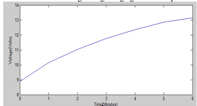
Fig. 6: Voltage graph of the Ultracapacitor during charging
