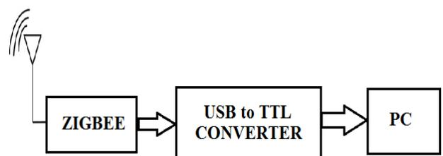
Fig. 2: Functional block diagram of the receiving system
