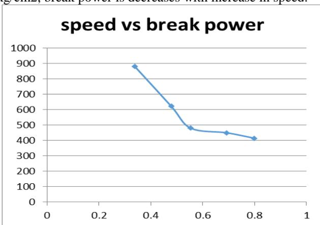
Fig. 5: Variations In Speed With Break Power
