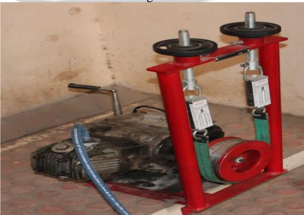
Fig. 3: Experimental Set Up For Air Engine with Modified Cam
