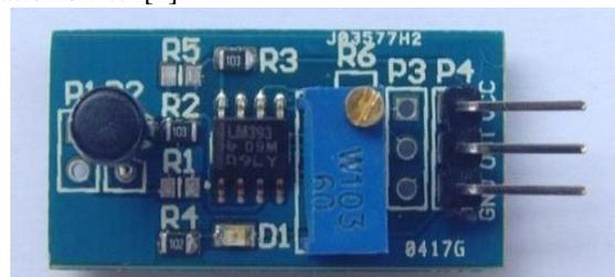
Fig. 7: Vibration Sensor
