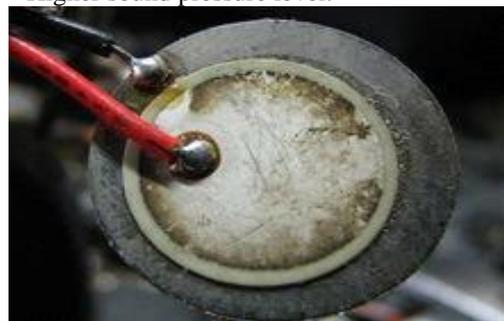
Fig. 11: Piezoelectric Buzzer
