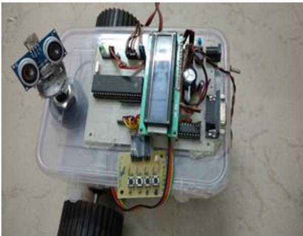
Fig. 5: Robot equipped with ultrasonic sensor
