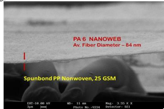
Fig. 1: Cross Sectional View of Electrospun Nanoweb Coated on Polypropylene Nonwoven (Adapted from [5]).
