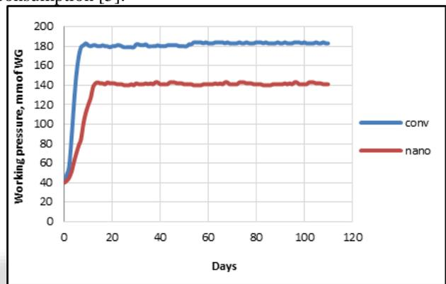
Fig. 2: Result of field trial in a paint industry with filter module made using nanofiber based media for dust filtration (Adapted from [5]).
