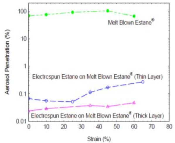
Fig. 8: Effect of deformation on aerosol penetration for melt blown Estane®, a thin layer of electrospun Estane®, and a thicker layer of electrospun Estane® on the melt blown substrate (Adapted from [17]).
