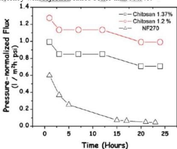
Fig. 3: Result of filtration performance of a three-tier Chitosan based nano filter against commercially available nano filter (Adapted from [7]).
