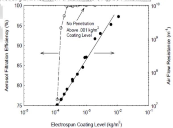
Fig. 9: Aerosol filtration efficiency and air flow resistance of open cell carbon-loaded foam as a function of electrospun fibre mass (Adapted from [17]).
