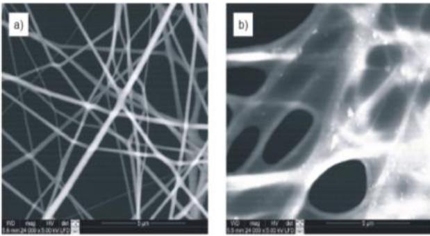
Fig. 7: Nano fiber membrane before (a) and after (b) filtering (Adapted from [16]).
