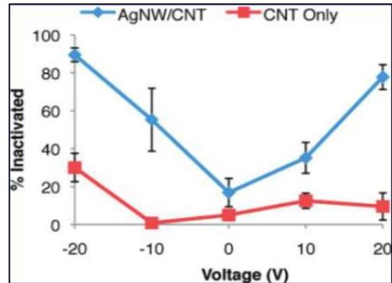
Fig. 6: Inactivation efficiency for AgNW/CNT cotton as well as CNT-only cotton (Adapted from [15]).
