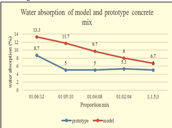
Fig. 3: Water absorption of model and prototype concrete mix
