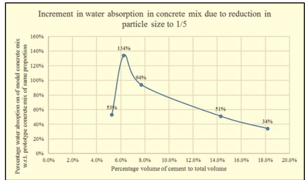
Fig. 5: Percentage increment in water absorption of concrete mix due to scaling
