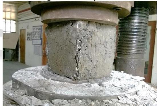
Fig. 1: Testing of concrete cube
