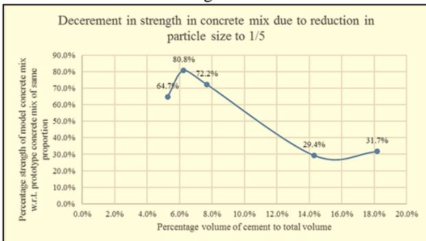
Fig. 4: Percentage decrement in strength of concrete mix due to scaling
