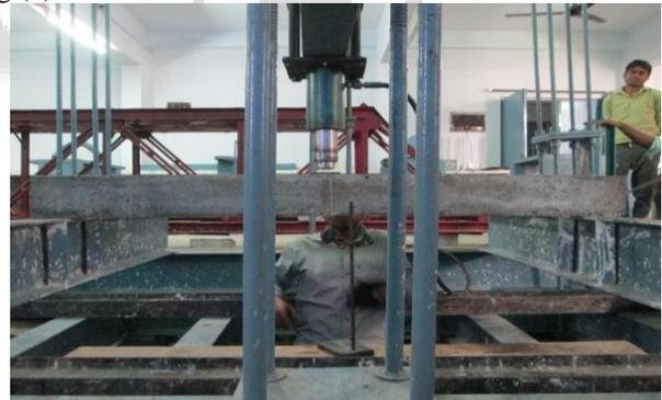
Fig. 3: Experimental Setup for Deflection Measurement
