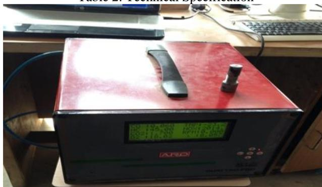
Fig. 2: Exhaust Gas Analyzer
