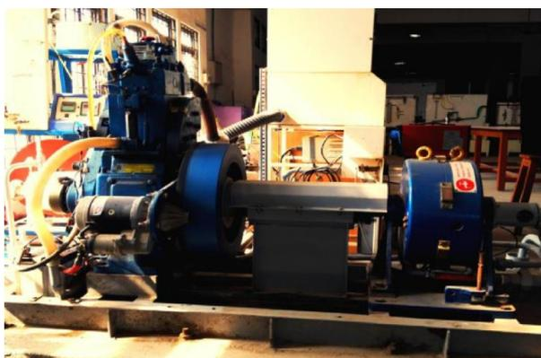
Fig. 1: Engine testing Rig(Trivedi, Patel, Patel, & Rathod, 2015)
