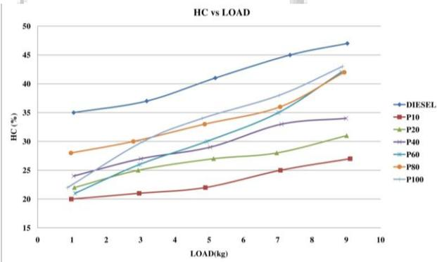
Fig. 3: Effect of various blends on hydrocarbons Emission
