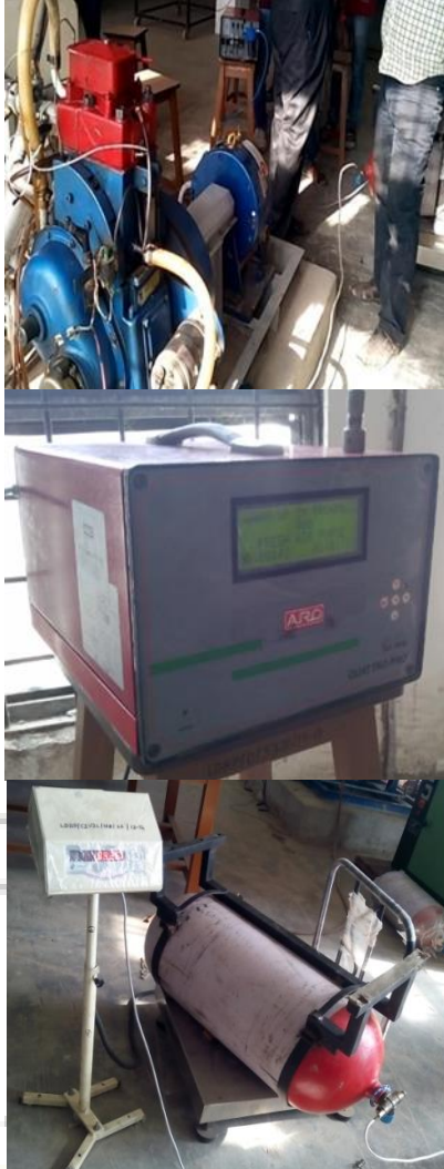
Fig. 1: Photo of experimental setup showing engine, gas analyser, Gas cylinder and weighing scale
