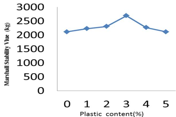
Fig. 9: Marshall Stability Value vs. Plastic Content
