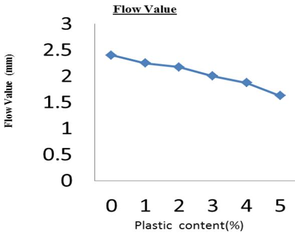
Fig. 10: Flow Value vs. Plastic Content
