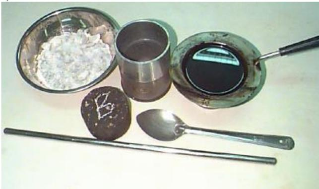
Fig. 2: Marshall Apparatus
