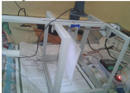
Fig. 5: Hardware Setup of Camera attached to Stepper Motor
