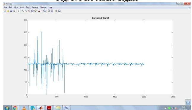
Fig. 4: Corrupted Audio Signal with Impulsive Noise
