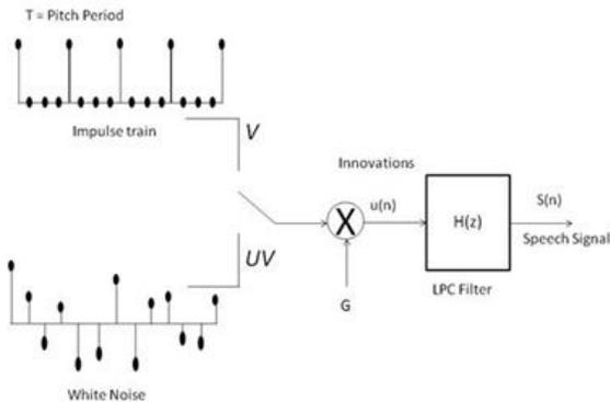
Fig. 1: Diagram For Synthesis Of Speech Signal
