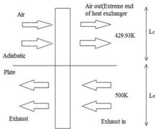
Fig. 4: One row of heat pipe heat exchanger.
