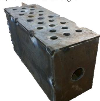
Fig. 6: Heat exchanger shell
