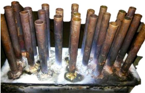
Fig. 7: Heat pipe inside the heat exchanger shell.
