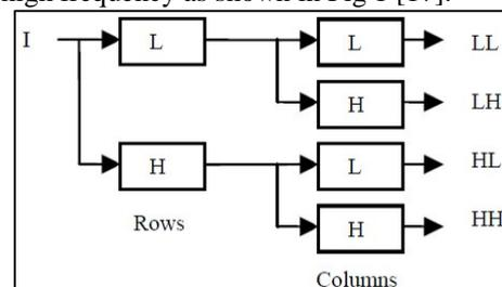
Fig. 1: Discrete Wavelet Sub-band Decomposition
