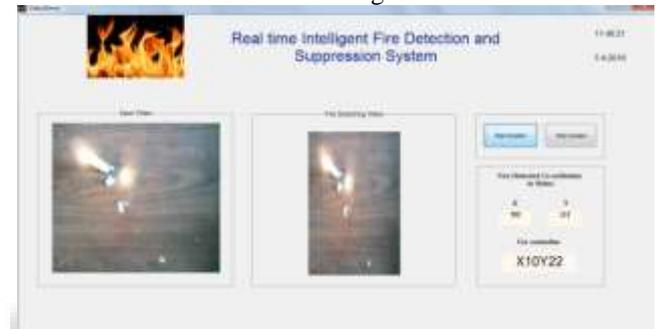
Fig. 5: Detection of fire and X-Y co-ordinate of fire
