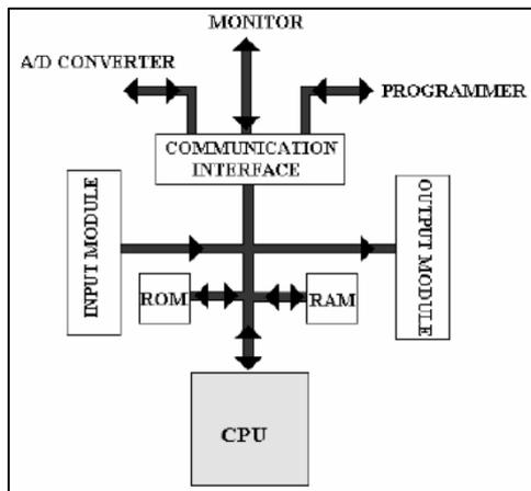
Fig. 2: PLC Architecture
