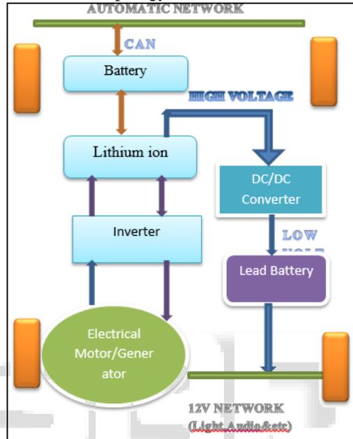
Fig. 8: Integrated Inverter/Converter multimotor drive system.
