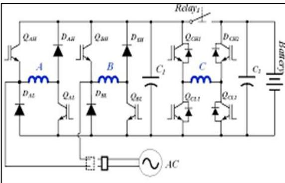
Fig. 2: Equivalent EV/HEV with integrated inverter circuit
