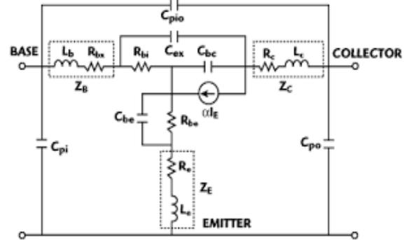
Fig. 13: small signal equivalent circuit
