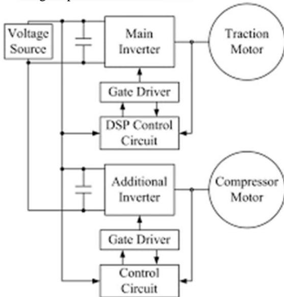
Fig. 7: Conventional Multi-motor Drive System
