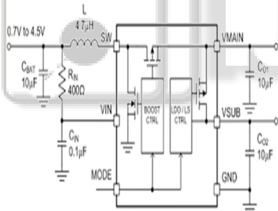
Fig. 10: Integrated circuit for dual mode of motor drives and boost converter
