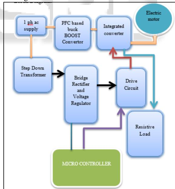
Fig. 10: Proposed Integrated Inverter/Convertor for the multi-motor drive system of EV/HE
