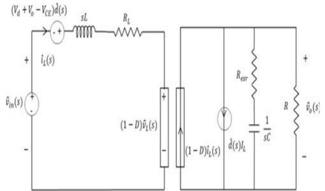
Fig. 3: Small signal equivalent circuit
