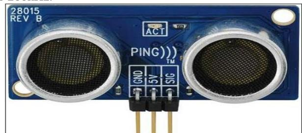
Fig. 7: Ultrasonic Sensor
