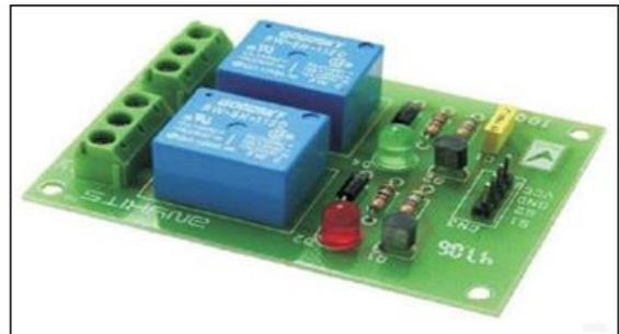
Fig. 6: Relay Driver Circuit
