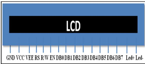
Fig. 8: LCD Pin Diagram
