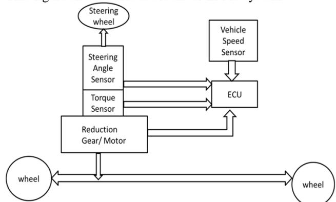
Fig. 2: Block Diagram of EPAS
