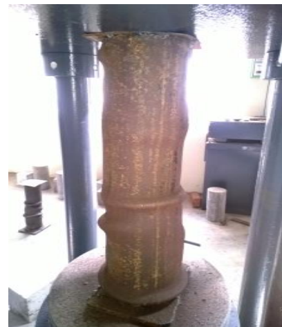
Fig. 2: Column 2- CFST containing 50% cement and 50% GGBS
