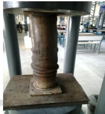
Fig. 3: Column 3- CFST containing 100% GGBS
