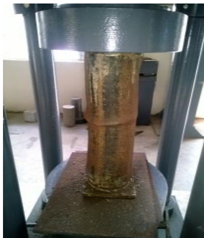
Fig. 1: Column 1- CFST containing 100% cement
