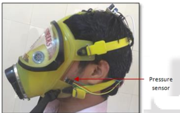
Fig. 5: Pressure Sensor Based Leakage Detection System
