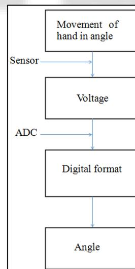
Fig. 3: Flow Diagram Of Transmitter
