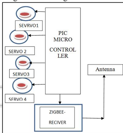
Fig. 2: Block Diagram Receiver
