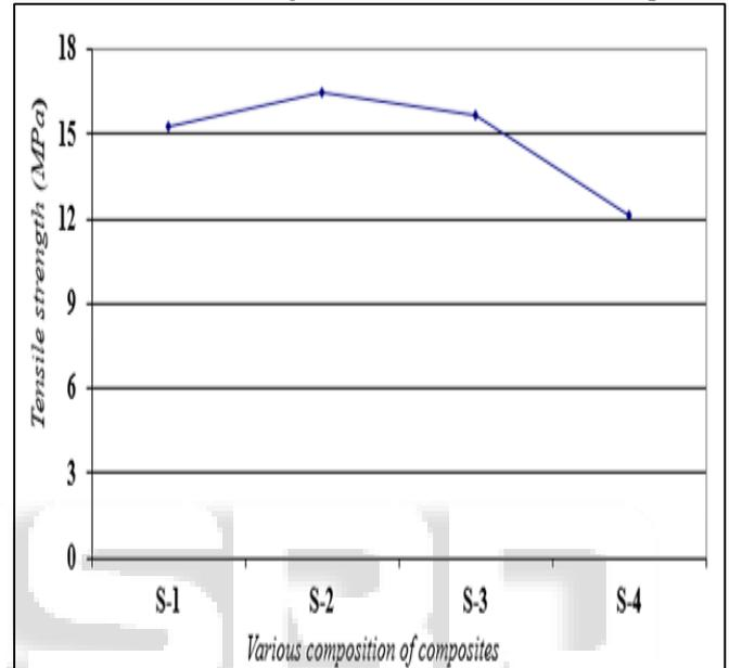
Fig. 4: Variation of Tensile strength for different composition of banana fiber epoxy composites
