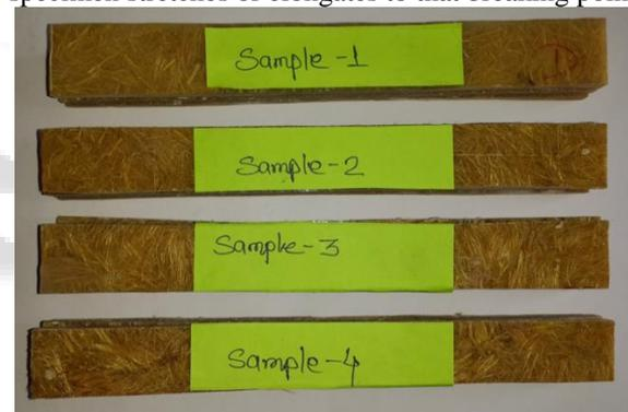
Fig. 1: Tensile test specimens
