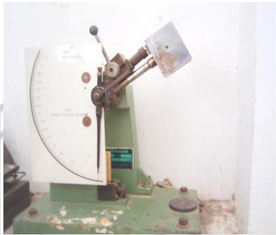
Fig. 3: Impact testing of the specimen
