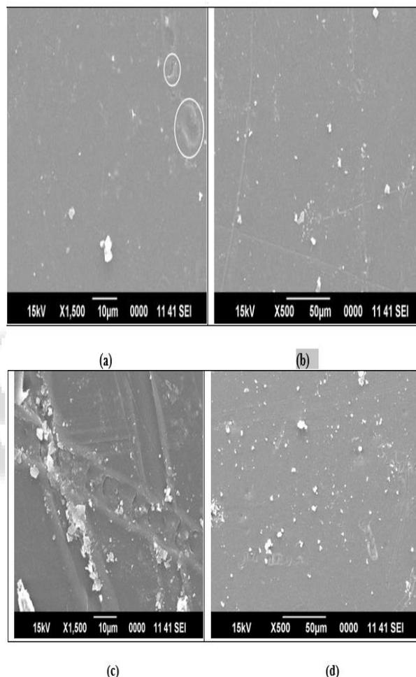
Fig. 8: Surface morphology of different composition of banana fiber epoxy composites.
