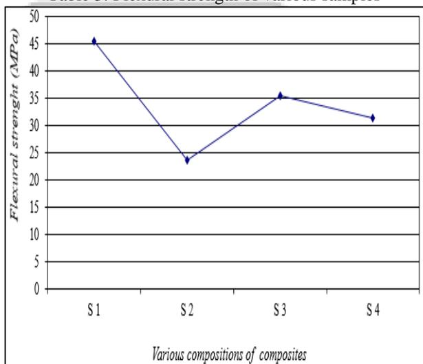
Fig. 5: Variation of Flexural strength for different composition of banana fiber epoxy composites
