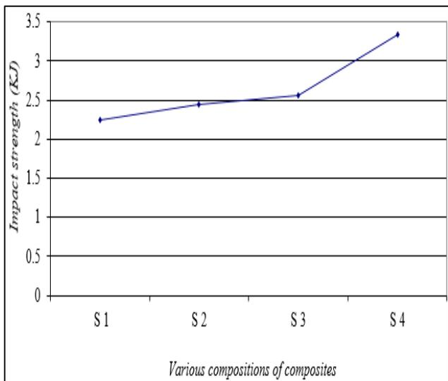
Fig. 6: Variation of Impact strength for different composition of banana fiber epoxy composites
