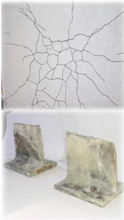
Fig. 11: Failure pattern of T connectors
