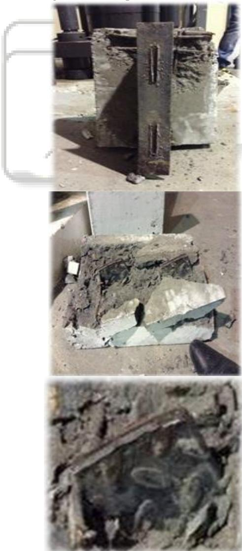
Fig. 12: Failure pattern of Embossed plate connectors
